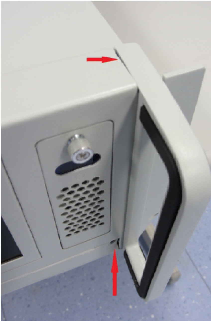
Figure 5: Bended handle right side and missing telescopic KBD/MS pad lock
