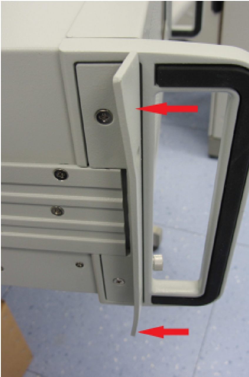
Figure 6: Bended rack mount flange left side
