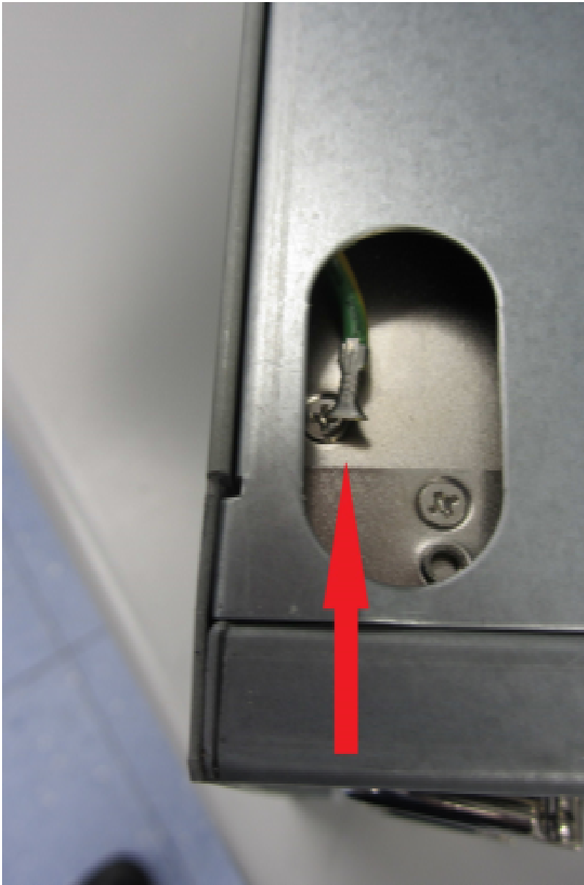
Figure 16: Broken safety earth connection
