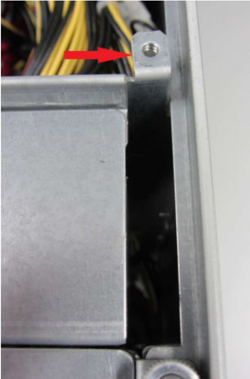
Figure 20: Misalignment of right internal top cover fixation
