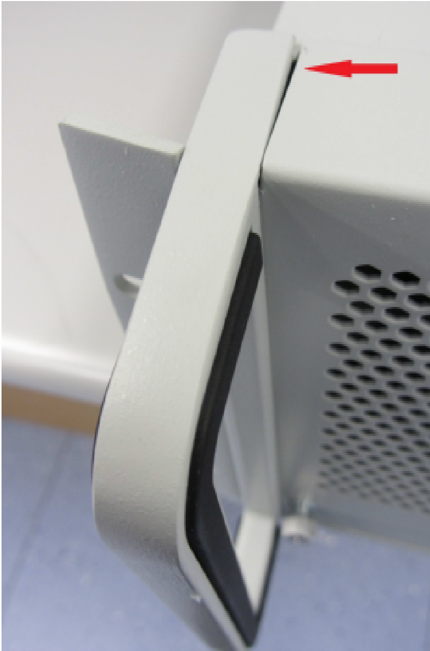
Figure 4: Bended handle left side
