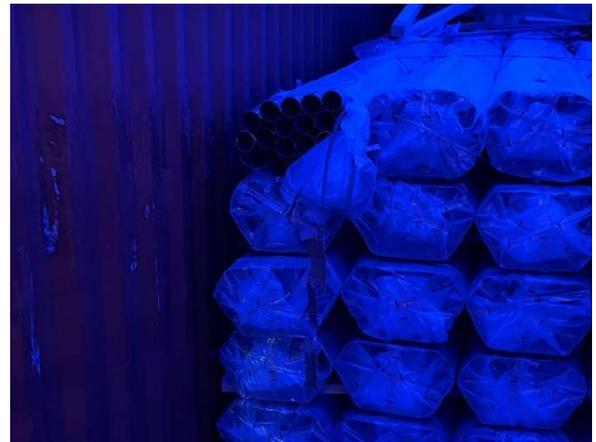
The tubes on the sides were obviously in contact with the wall. The film was open on one bundle, and a laterally deformed tube was visible.
