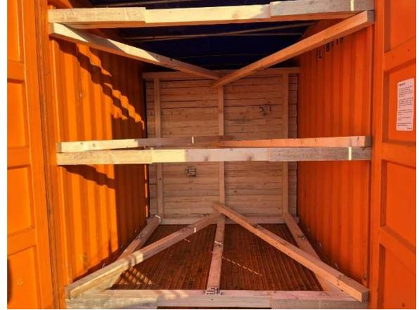
The load could be inspected via the wooden wall. It was seen that the bundles of tubes were stowed five layers high with four bundles per layer. Timber had been used as intermediate layers and had been lashed down with belts over the top layer.
